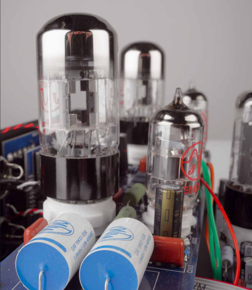
On the left, one of the two 6SN7 and, in front of it, the E88CC. Both are double triodes, and the latter is a tension grid tube. You can hear the difference clearly
