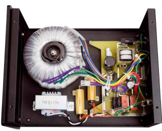
The external power supply with transformer, choke coil and rectifier circuit
