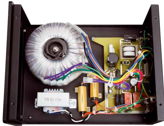
The external power supply with transformer, choke coil and rectifier circuit
