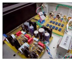
Situated right in device, there is another power supply board for voltage regulation; behind it is a whole bank of relays to switch the gain stages
